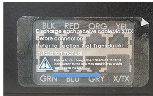
Figure 14. DRX with the Transducer Receive Discharge cover label instruction
