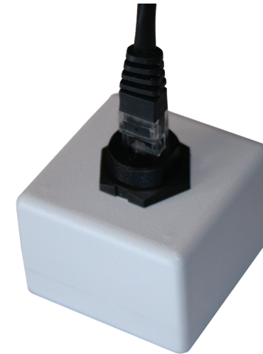
Figure 16. Discharging Transducer Channels
