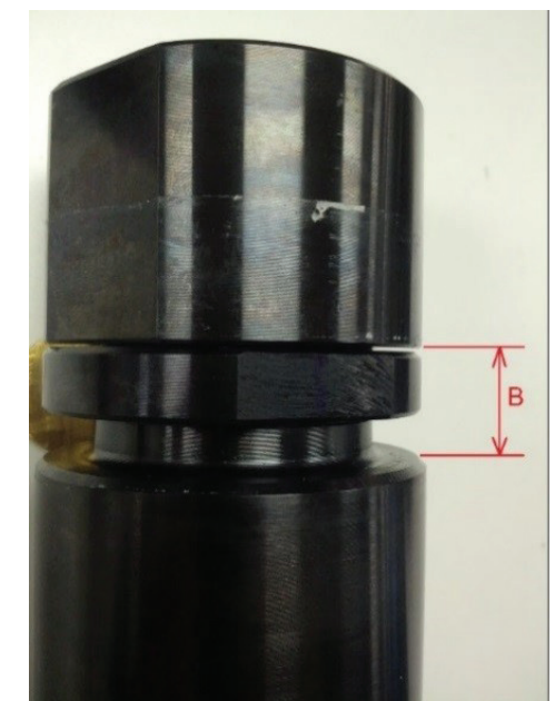
Figure 12. Gland nut travel measurement point for steel glands
